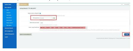
> Interface Configuration > Mode Select "Client", double check ESSID and Wireless Security (Key) is correct, click SAVE & APPLY button.
