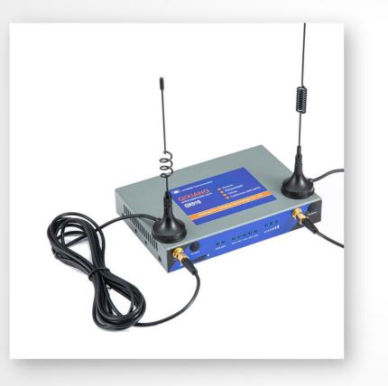
// QX510 Industrial grade cellular LTE Cat 4 router with rugged metal housing is a compact and easy to use connectivity device that can provide cellular capabilities to equipment across all market segments.
