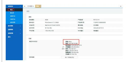
If the IP address is not as of xxx.xxx.xx.248, you have to manually set static IP address for Service WAN port as following:
